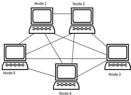
**Fully-connected mesh network** 필요.
